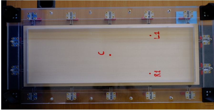
Figure 2: Schematic representation of the measurement setup. The red dots L1 and C indicate the excitation points, namely locations for either the impact hammer hits or the contact point for the exciters while performing the validation measurements, while R1 indicates the position of the accelerometer.
