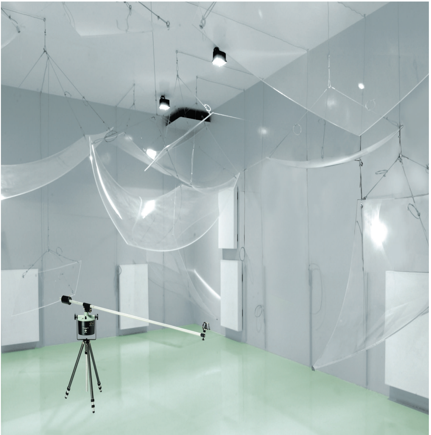
Figure 3 Rotating boom in reverberant chamber with acoustic diffusers
