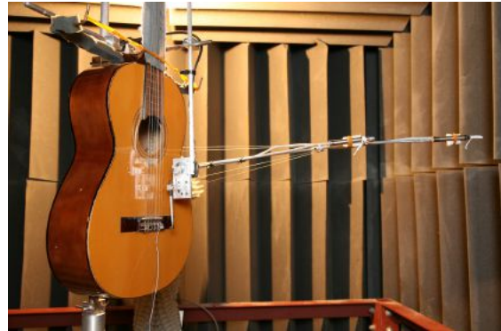
Figure 2: The anechoic chamber at Cardiff in use for the measurement of sound fields and radiation efficiency.
